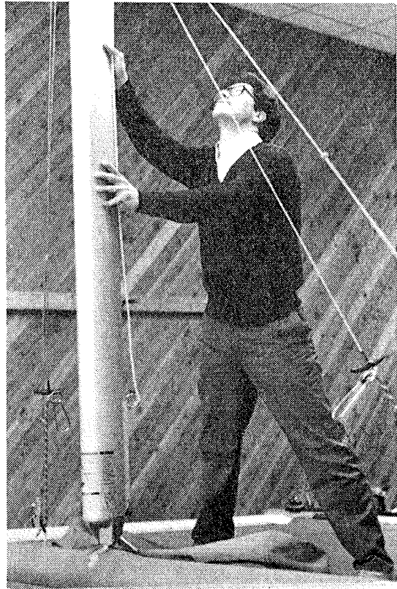
Photo J2. Proper stance for lowering the mast.
