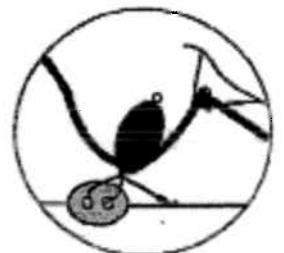
H-25 Tie line through rear crossbar and cap and around bolt. Fasten to block. Hook halyard to trampoline lace line to hold block from water.
