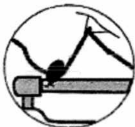
H-16 Shunt eye strap to rear end of wire halyard. Shackle block to eye strap. Twist on spring as though putting key on key ring. Spring holds block in upright position.
