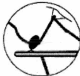
H-21 or H-22 Shunt eye strap to outboard and rear of wing tube. Shackle block to eye strap. Twist on spring as though putting key on key ring. Spring holds block in upright position.
