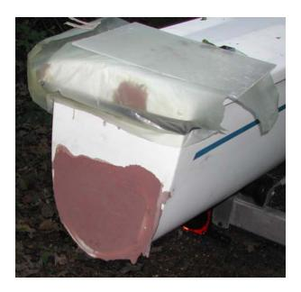
**Drill mounting holes and finish the drain port.** Drill 1/16<sup>th</sup> pilots into where the gudgeon mounting holes should be, using the upper one to locate the lower one, with rudder pin in between them. Adjust locations as the hole size is increased to 5/32". Run a #12-24 tap through the 8 gudgeon holes. Finish the drain port, making sure the plug base fits snugly.
