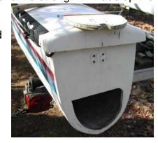
Sandwich the cutout between thick, flat plastic and clamp down with several clamps, starting the center and working to the edges to squeeze out air. Wood boards on each side can stiffen the clamp effort. Wipe off excess epoxy, down to the core cutout material. Let cure overnight, finish side down, in a warm area where the odor won't bother anyone.
