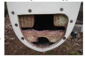
because there is no clamping to hold the strips in place. The extra epoxy filled remaining gaps. Wipe excess from the edges of the opening and the front surface of the blocks.
