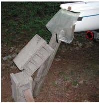
I tried holding a piece of 3/16" polyethylene plastic sheet against the epoxy using blocks and a 2X4 to hold it in place. It helped reduce filing and finishing.
