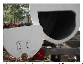
Cut the transom section out with a coarse-bladed reciprocating saw. Save the piece to put it back in later. Be careful to retain the steel plate in its original location, so the gudgeon screws will line up again.
