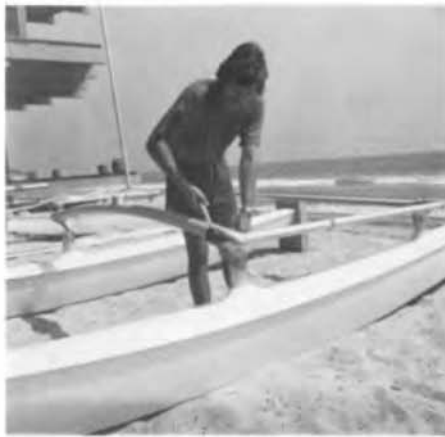
2 Coat the corner pylons with a generous amount of white grease or vaseline. Carefully place and balance the wing section on top of the four corner pylons (an assistant is most helpful).
