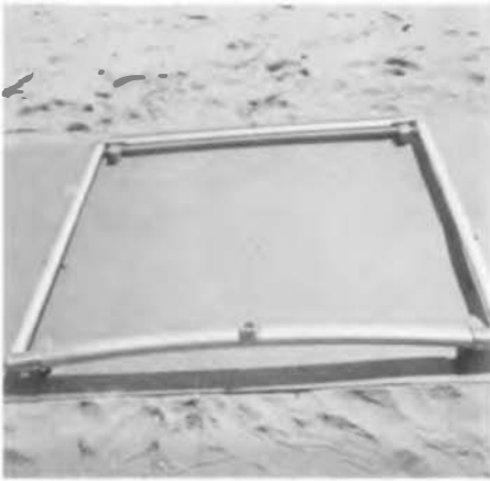
1 Assemble the wing section noting that the grooves in the side bars are in the front facing inside, and chain plates are on outside.
