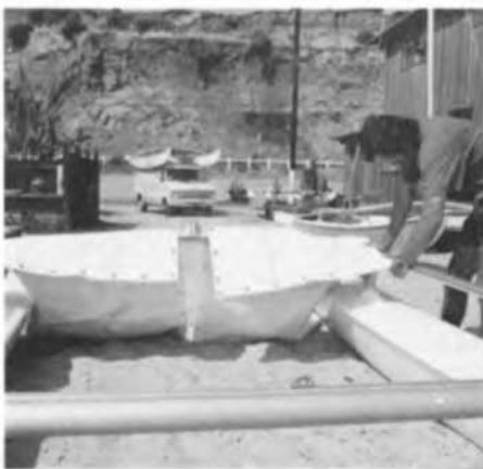
7 Lay both trampoline halves over the front cross-bar noting that the grommets run down the center and along the rear.
