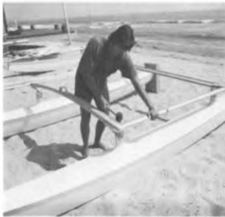
5 Beginning again at the front left casting, rubber mallet the casting all the way down until the holes line up. CAUTION: Strike the casting on the flat portion directly over the pylon only.
