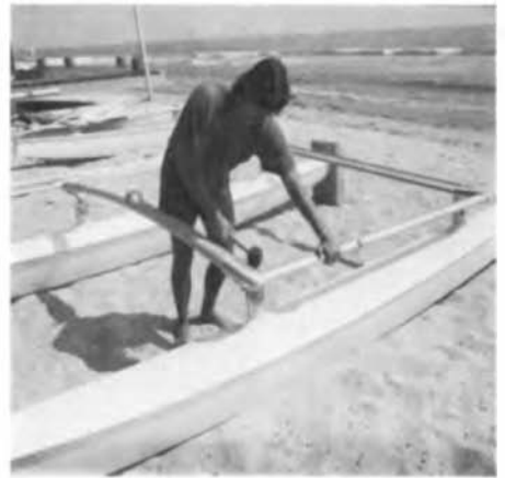
3 Beginning at the front left, line up the corner casting with pylon by using a rubber mallet and gently tapping forward and side edges. Once it is lined up, tap the casting down only part way on the pylon.
