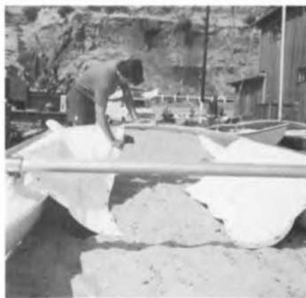
8 Insert the trampoline into the groove on the forward inside of the side bars. Gradually feed them back all the way to the rear. Next, insert the front of the trampoline into corner slot in the front crossbar and feed them all the way to the center.
