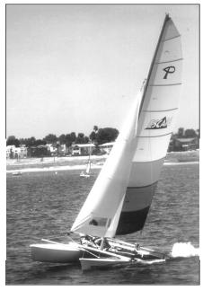
need for daggerboards, which makes the Escape an ideal beach boat. Powering the Escape is a modest sized sailplan and self-furling jib. The boomless rig and lack of mast spreaders also help to eliminate weight and add sailing comfort.
